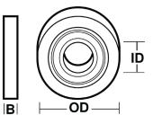
BARCODE: 9314350013728 OD DIAMETER: 16mm ID DIAMETER: 5mm DEPTH: 5mm QUANTITY: 1 WEIGHT: 5g
