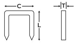
LENGTH: 12mm CROWN: 10.8mm THICKNESS: 1.25mm
