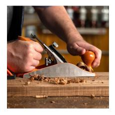
BARCODE: 044295707305 LENGTH: 255mm (10") WIDTH: 64mm BLADE LENGTH: 177mm BLADE WIDTH: 50mm BLADE THICKNESS: 3mm WEIGHT: 1941g
