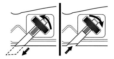
Insert a new blade into the cutter groover, install the new blade by turning the thumbwheel counter-clockwise.
