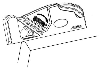
Advance the blade by turning the thumbwheel clockwise (when viewed from the top) until the blade is in contact with the wood.
