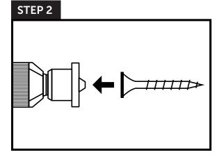
**Position the Screw**: Place the screw onto the screw guard. It's magnetic feature should hold the screw in place.
