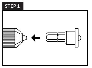
**Insert the Screw Guard:** Attach the screw guard to the drill chuck, ensuring it is secure.
