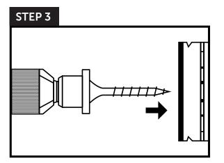
**Drive the Screw**: With steady pressure, drive the screw into the plasterboard.
