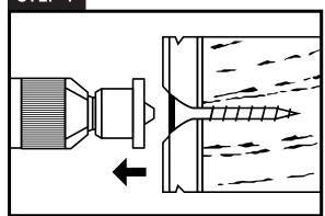
Secure the Screw: Continue driving the screw until it reaches the required depth.
