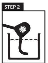
All air pockets must be expelled from the intage hose. Full length of intake hose must be fully submerged before starting pump.
