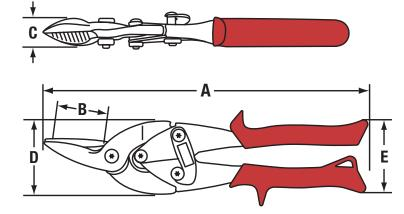
BARCODE: 727226130662 OVERALL LENGTH (A): 254mm CUTTING EDGE (B): 31.8mm JOINT THICKNESS (C): 20mm JOINT WIDTH (D): 57mm HANDLE SPAN (E): 50mm COLOUR: Red BLADE PATTERN: Left WEIGHT: 410g
