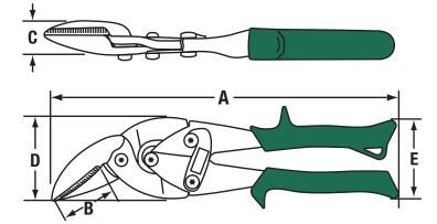
BARCODE: 727226130327 OVERALL LENGTH (A): 247.7mm CUTTING EDGE (B): 31.8mm JOINT THICKNESS (C): 27mm JOINT WIDTH (D): 57mm HANDLE SPAN (E): 50mm COLOUR: Green BLADE PATTERN: Right WEIGHT: 430g
