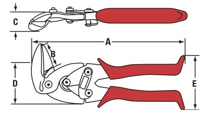
BARCODE: 727226130709 OVERALL LENGTH (A): 203.2mm CUTTING EDGE (B): 31.8mm JOINT THICKNESS (C): 24mm JOINT WIDTH (D): 57mm HANDLE SPAN (E): 50mm COLOUR: Red BLADE PATTERN: Left WEIGHT: 450g
