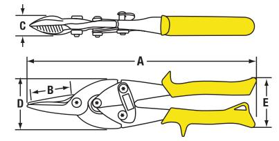
BARCODE: 727226130686 OVERALL LENGTH (A): 254mm CUTTING EDGE (B): 34.9mm JOINT THICKNESS (C): 20mm JOINT WIDTH (D): 57mm HANDLE SPAN (E): 50mm COLOUR: Yellow BLADE PATTERN: Straight WEIGHT: 390g
