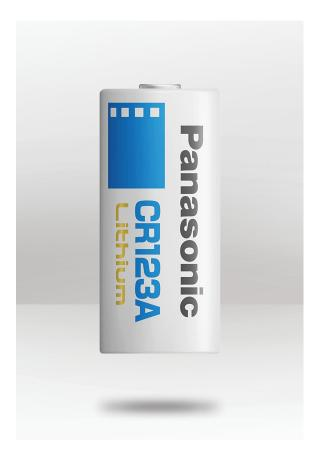
BARCODE: 4984824348554 MODEL: CR123A NOMINAL VOLTAGE: 3V NOMINAL CAPACITY: 1550mAh CONTINUOUS DRAIN: 20mA DIAMETER: 17mm HEIGHT: 34.5mm MASS: 16g QUANTITY: 1 PACKAGING DIMENSIONS: 92 x 112 x 18mm
