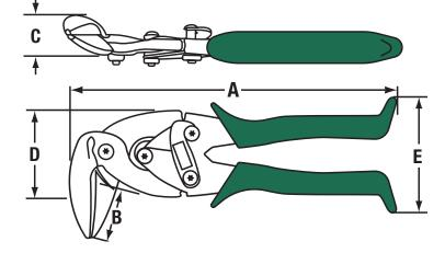
BARCODE: 727226130716 OVERALL LENGTH (A): 203.2mm CUTTING EDGE (B): 31.8mm JOINT THICKNESS (C): 24mm JOINT WIDTH (D): 57mm HANDLE SPAN (E): 50mm COLOUR: Green BLADE PATTERN: Right WEIGHT: 450g
