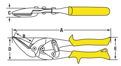
BARCODE: 727226130655 OVERALL LENGTH (A): 247.7mm CUTTING EDGE (B): 38.1mm JOINT THICKNESS (C): 27mm JOINT WIDTH (D): 57mm HANDLE SPAN (E): 50mm COLOUR: Yellow BLADE PATTERN: Straight WEIGHT: 450g
